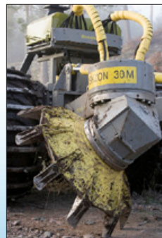
Discs with replaceable teeth.
