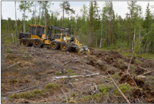
The Bracke T26.b is mounted on a medium-sized or large prime mover.
