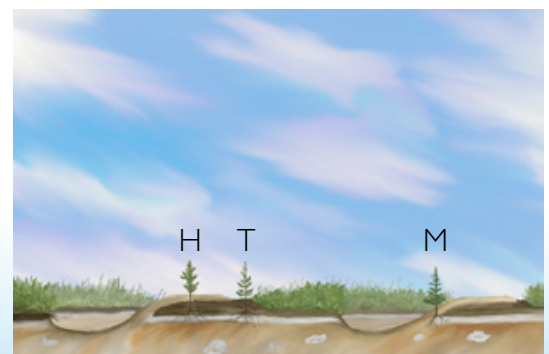
The Bracke M36.b creates planting spots with inverted humus (T), mineral soil mounds on inverted humus (H), and mineral soil mounds (M).
