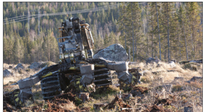
The Bracke T35.b is suitable for large scarification objects and is mounted on large prime movers.
