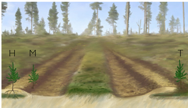
The Bracke T35.b creates planting spots with inverted humus (T), mineral soil mounds on inverted humus (H), and mineral soil mounds (M).
