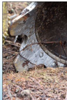
Discs with replaceable teeth.
